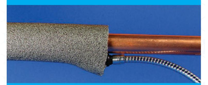
An insulated pipe being scanned for leakage. It is important that the insulating material is not glued to the metal pipe and does not have any open gaps or tears.
