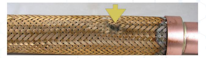
The faint dark area on this vibration eliminator is evidence of oil-refrigerant seepage.
