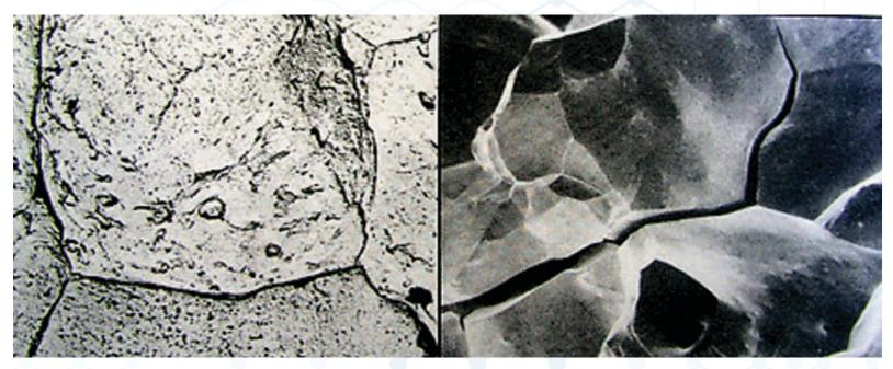
An electron micrograph of a "clean" silver soldered joint. Note the crack lines and other impurities of the melted metal.
