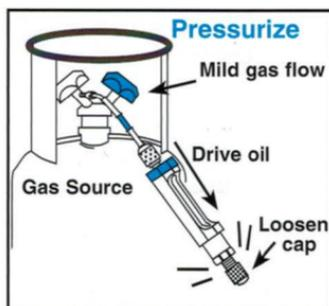
6. Stop flow by tightening the flare cap and close the gas valve.
