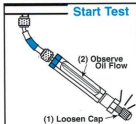
7. As soon as the Oil hits the Indicator, stop flow immediately by tightening the flare cap. Close the suction port.
