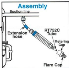
4. While the system is running, loosen the flare cap to commence a s-l-o-w bleed.
