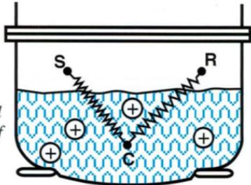
The ideal Oil should be nonconductive however, even virgin Refrigeration Oil will register slight conductivity. Working Compressor Oil will manifest conductance due to chemical interaction, notwithstanding, the introduction of contaminants during an installation or repair.
